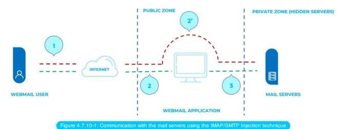
Figure 1 depicts the flow of traffic generally seen when using webmail technologies. Step 1 and 2 is the user interacting with the webmail client, whereas step 2 is the tester bypassing the webmail client and interacting with the back-end mail servers directly.
